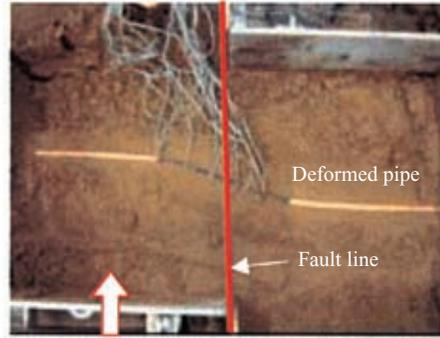
Fig.5 Bending of a buried pipeline due to shear deformation
