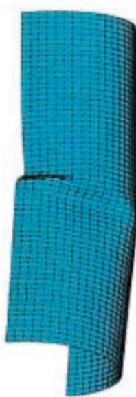
Fig.4 Shell wrinkling due to bending
